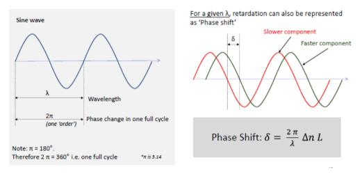
Figure 10: Diagrammatic representation of retardation as a "phase shift"
