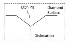
Figure 7: Cross-section of an etch pit
