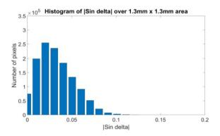
Figure 15: Histogram of  $|\sin \delta|$  over 1.3mm x 1.3mm area for Sample 3
