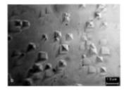
Figure 6: Etch pits on diamond with dislocation density of 3300/mm<sup>2</sup>
