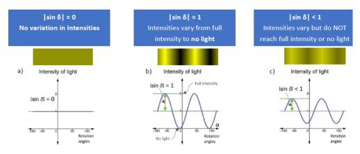
Figure 11: Graphs depicting the variation of intensities of light against the polariser's Rotation Angle
