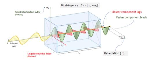
Variation in 'n' forces light to split into two components along fastest and slowest axes Figure 9: Diagram showing how the variation in the refractive index causes birefringence
